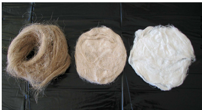
Fig.3 Left: unbleached flax; Middle: bleached flax (using POM catalysts); Right: bleached flax following alkali extraction.
