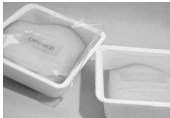
Fig. 5 Oxygen indicator detecting leak [30, 31]
