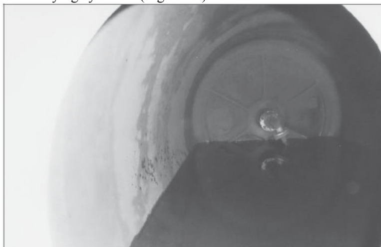
Fig. 24. Inner appearance of cylinder, with condensate
