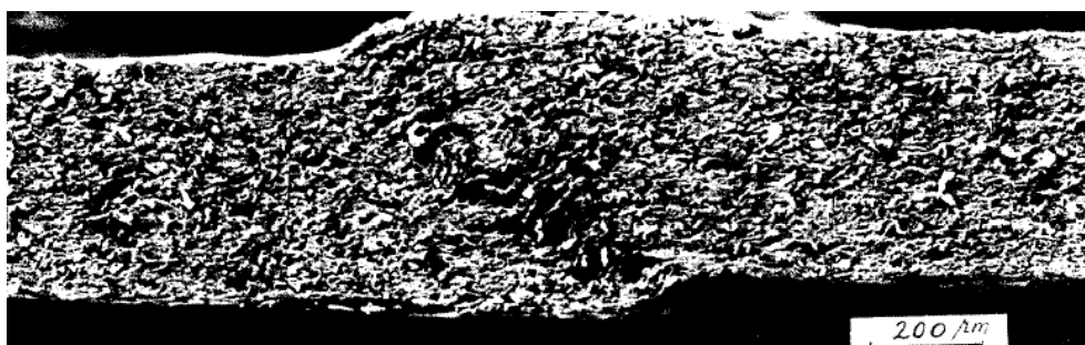
Fig. 1 Shear dislocation type of failure of a 300 g/m 2 linerboard subjected to SCT testing
